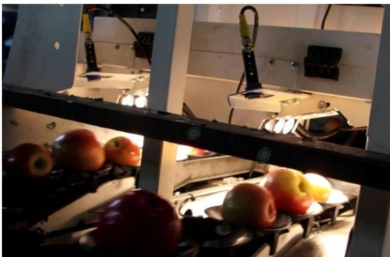
**Figure 7a.** On line detection of internal browning in apple (IDD unit from CVS-MAFRoda).
